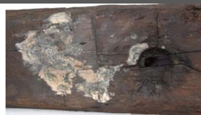
The sulfurated "leprosy" on wood treated with PEG: Collection Villefranche/Sea Lomellina, Genoese wreck of the 16 th century
