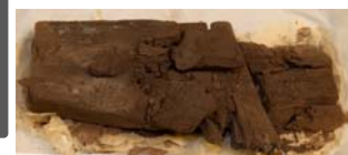
A fragment considered one of the worst case of alum-treated wood from the Oseberg finds
